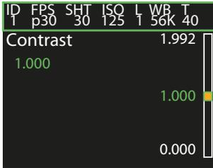
Set contrast with navigation and ENTER button. The orange mark in the sidebar is what you want to select. Your previous setting is displayed in green. Contrast can be set in steps of 0.008 from 0.000 to 1.992.
